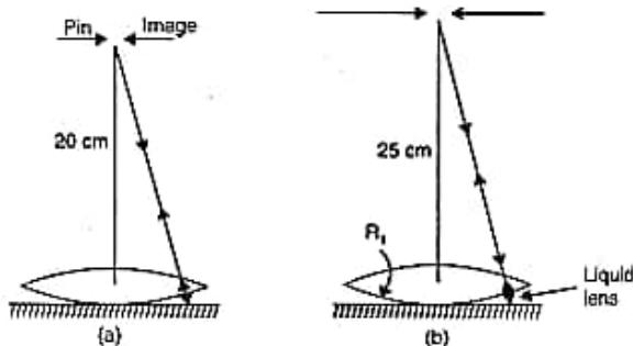
In the first case, the image will coincide with the pin if the rays from the pin, after refraction through the lens, fall normally on the mirror and retrace their path, as shown in fig (a). This means that the focal length of the convex lens is 20 cm, i.e.  $f_1 = 20 \text{ cm}$
