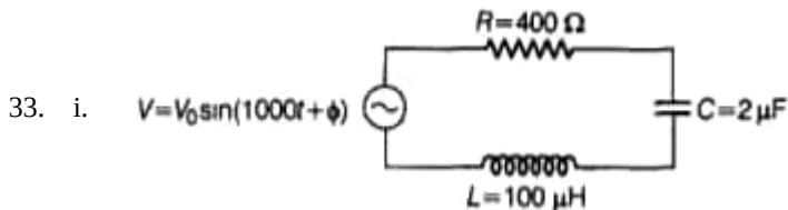
$$V = V_0 \sin(1000t + \phi) \Rightarrow \omega = 1000 \text{ Hz}$$
