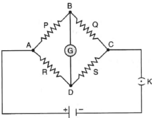
Galvanometer G is connected between points B and D and battery B is connected between A and C. Now in the balance condition, when the deflection in the galvanometer is zero in the closed mesh ABDA, then by applying Kirchhoff's law,
