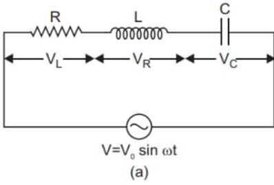
Suppose the voltage across resistance R is  $V_R$ , voltage across inductance L is  $V_L$  and voltage across capacitance C is  $V_C$ . The voltage  $V_R$  and current  $i$  are in the same phase, the voltage  $V_L$  will lead the current by angle  $90^\circ$  while the voltage  $V_C$  will lag behind the current by angle  $90^\circ$ . Clearly  $V_C$  and  $V_L$  are in opposite directions, therefore their resultant potential difference  $= V_C - V_L$  (if  $V_C > V_L$ ).
