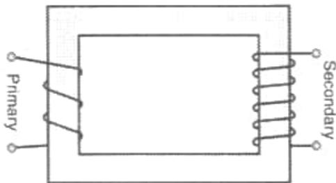
$$\text{Input power, } P_i = I_i \times V_i = 15 \times 100 = 1500 \text{ W}$$
