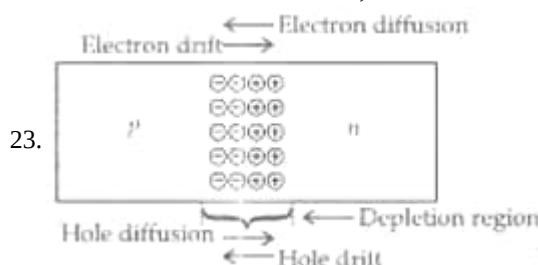
Due to the diffusion of electrons and holes, from their majority to minority zone, a layer of positive and negative space charge region on either side on the junction is formed. This is called the depletion region. The loss of electrons, from the n-region and the gain of electrons by the p-region, cause a difference of potential across the junction formed. This tends to prevent the further movement of charge carriers across the junction and is, therefore, termed as barrier potential.
