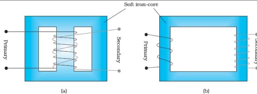
**Working:** When an alternating voltage is applied to the primary, the resulting current produces an alternating magnetic flux which links with the secondary and induces an e.m.f. in it.
