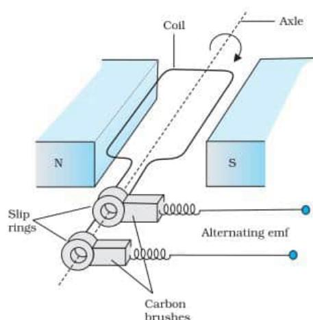
**Construction** – It consists of a coil placed in a magnetic field. The coil is mounted on a rotor shaft. The ends of the coil are connected to an external circuit by means of slip rings and brushes.
