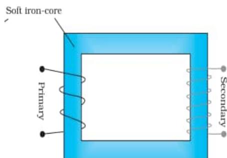
**Working** - when an alternating voltage is applied to the primary, the resulting current produces an alternating magnetic flux which links the secondary and induces an emf in it.
